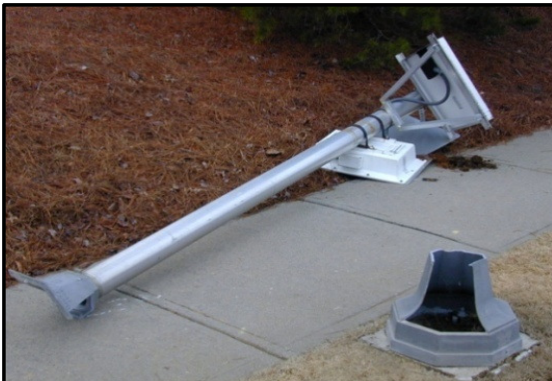
The radar sign sustained minimal cosmetic damage to the YOUR SPEED faceplate. The radar sign and solar panel remained operational and intact.
