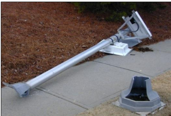
The radar sign sustained minimal cosmetic damage to the YOUR SPEED faceplate. The radar sign and solar panel remained operational and intact.
