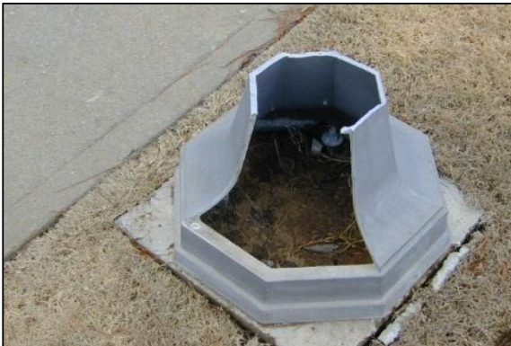
Radarsign's pole base broke away from the sign pole on impact as it was designed to do.
