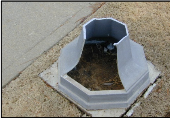
Radarsign's pole base broke away from the sign pole on impact as it was designed to do.
