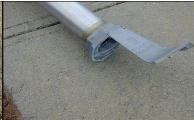
Radarsign's pole base broke away from the sign pole on impact as it was designed to do.
