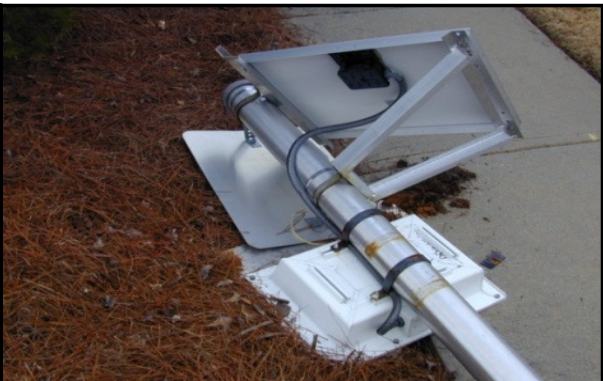
The radar sign sustained minimal cosmetic damage to the YOUR SPEED faceplate. The radar sign and solar panel remained operational and intact.
