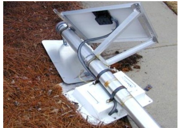
4.) The radar speed sign sustained minimal cosmetic damage to the YOUR SPEED faceplate. The radar speed sign and solar panel remained operational and intact.
