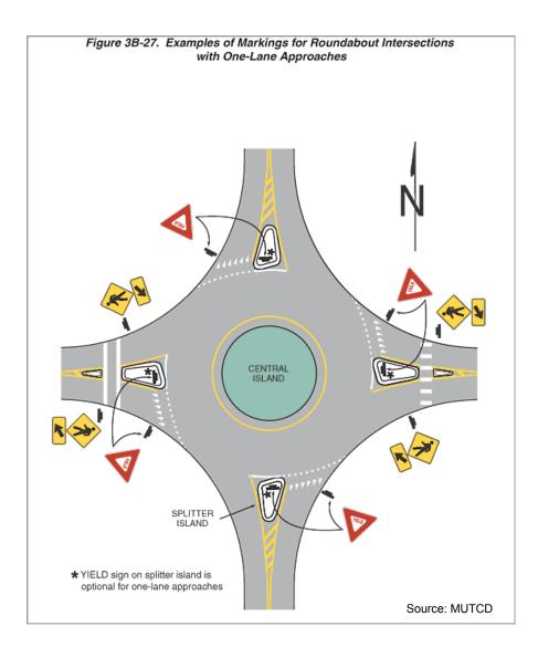
The figure shows a central island surrounded by a circular roadway, which is created with four streets that enter/exit the roundabout. Triangular splitter islands separate oppositional traffic directions. Markings include:
