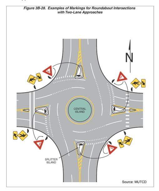
Markings for the two-lane entry roundabout are the same as those for the one-lane entry with one addition:
