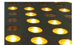
Individual cones for each LED
