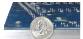
3/8" Bashplate protects LEDs
