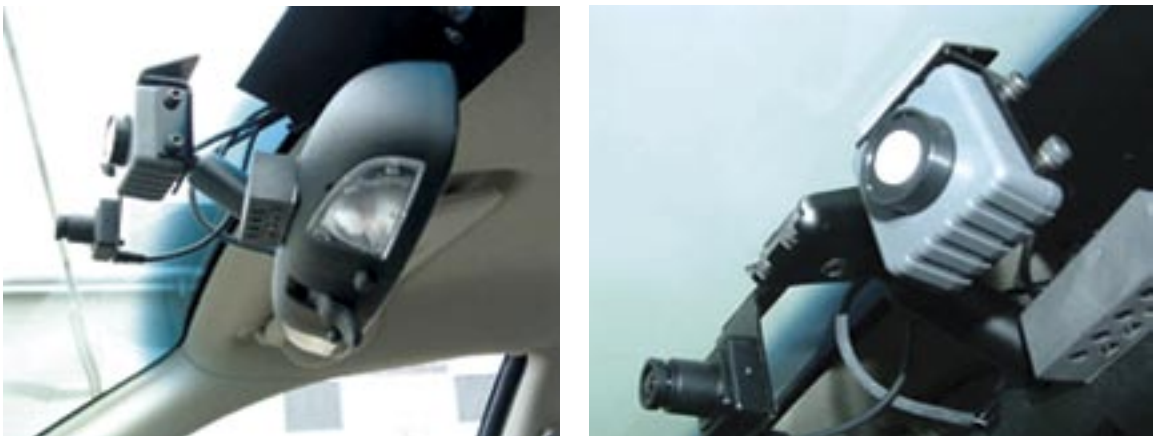
Figure 7. The mounting for the glare sensor behind the rearview mirror. The forward-view camera was part of the same mounting assembly.
