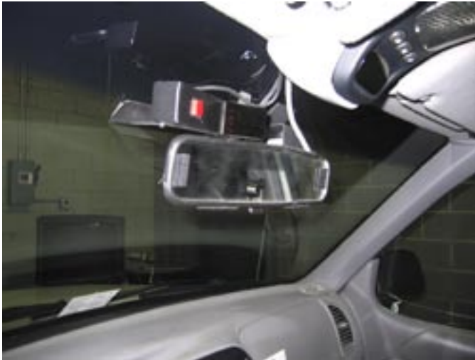
Figure 6. The incident pushbutton box mounted above the rearview mirror. The right-hand portion contains the driver-face/left-road view camera hidden behind a smoked plexiglas cover.
