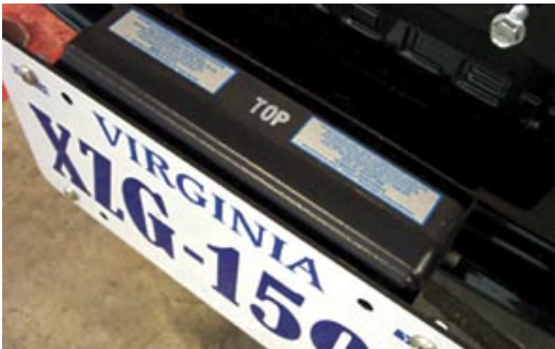
Figure 5. Doppler radar antenna mounted on the front of a vehicle, covered by a plastic license plate.
