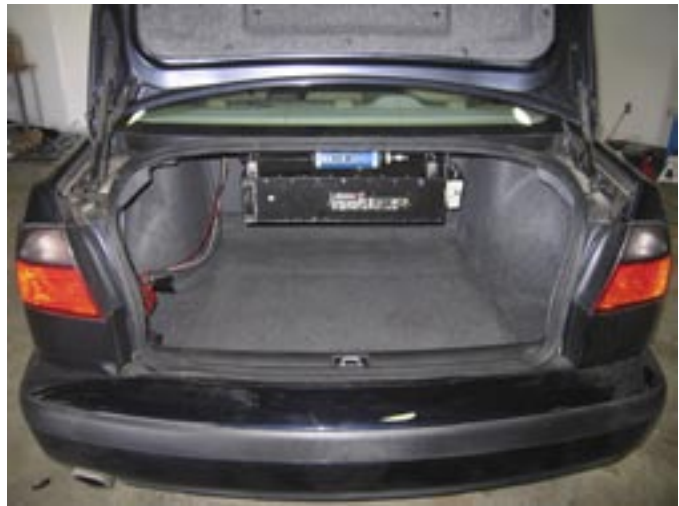
Figure 4. The main DAS unit mounted under the trunk “package shelf.”
