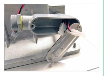
Take the two pairs of wires that are inside of the conduit and feed them into the junction box.
