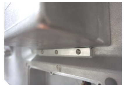
Bottom of battery / AC accessory housing with ridge seated in the sign housing ledge
